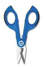
The tool is suited for dismantling and stripping Cu/Al conductors as well as crimping wire ends between 0.5 and 4 mm<sup>2</sup>. The stainless blades are made of high-quality INOX steel (hardened to 55 HRC) which makes them very durable. Due to fine micro toothing on the blades of the scissors, very precise flush and non-slipping cutting is made possible. The non-slip 2-component handles made of impact resistant fiberglass reinforced plastic ensure safe working.
