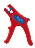
The WEICON Wire Stripper No. 6 has an adjustable length stop from 5 - 12 mm. This allows all flexible and solid conductors of 0.2 - 6.0 mm² (24 - 10 AWG) to be stripped. The length stop can be removed if required. This fully-insulated tool is subject to routine testing in accordance with the VDE regulation as per IEC 60900:2004 and can withstand a voltage of 1000 volts.
